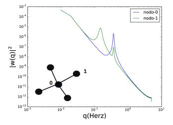
Fig. 2. Frequency signal power spectrum, for two nodes in a power grid with star topology.
